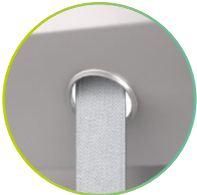
1 Flanged guide holes. The flanged guide holes protect the lift tape from damage from sharp punched hole edges, to ensure its problem-free operation and long service life.
